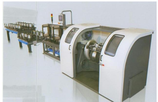
Take up bobbins diameters from 250mm up to 1250mm
