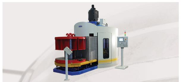
The Teurema EVM Automatic Spooler can handle a 3.5mm to 16mm wire range at a speed of 16 m/s
