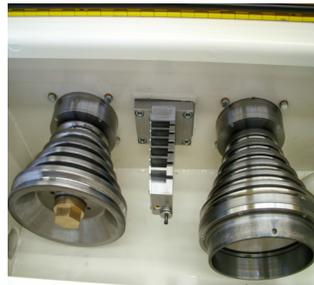
Fig. 1 Cone Type Wet Drawing Machine
